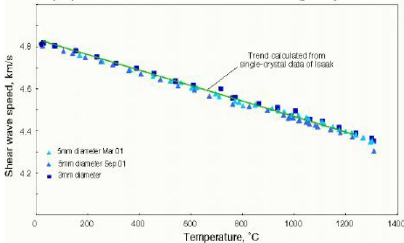
Comparison of measurements performed on  $Fo_{90}$  specimens of two different diameters (5 and 3 mm) indicating the insensitivity of the results to the size of the specimen and also the close approach to the temperature dependent modulus calculated from single-crystal elasticity data.
