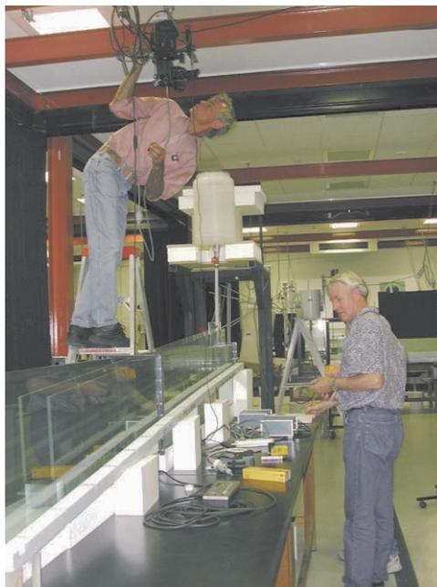
*Figure 1:* Work in the recently opened Geophysical Fluid Dynamics laboratory, showing apparatus being used to study cooling and solidifying channel flows and the dynamics of basaltic lava channels.
