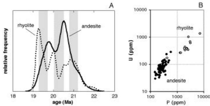
Figure 6: Age spectra (A) and trace element compositions (B) of zircons in andesite and rhyolite porphyries from the Kelian gold deposit.
