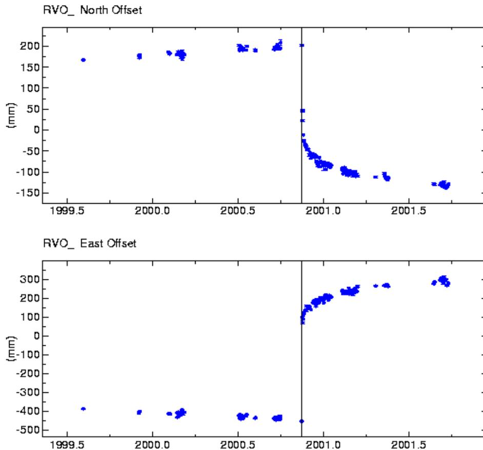
*Figure 1:* Time series of in local north and east coordinates of the position estimates at the Rabaul Volcano Observatory continuous GPS site with respect to the rigid South Bismarck Plate. Co-seismic offsets and the post-seismic relaxation are clearly evident.
