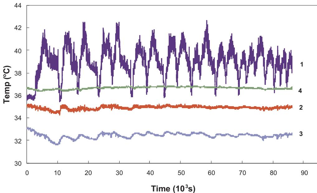
Figure 5: An example of temperature records from the laboratory experiment with thermal and salinity buoyancy fluxes in a ratio that leads to oscillatory behaviour. Three records shown are from thermistors fixed 1cm above the base in the bottom boundary layer of the flow and (1) within the warm, salty bottom layer near the salt input, (2) at the centre of the heated base, (3) at the centre of the cool base. Record (4) is from the flow near the top of the tank.
