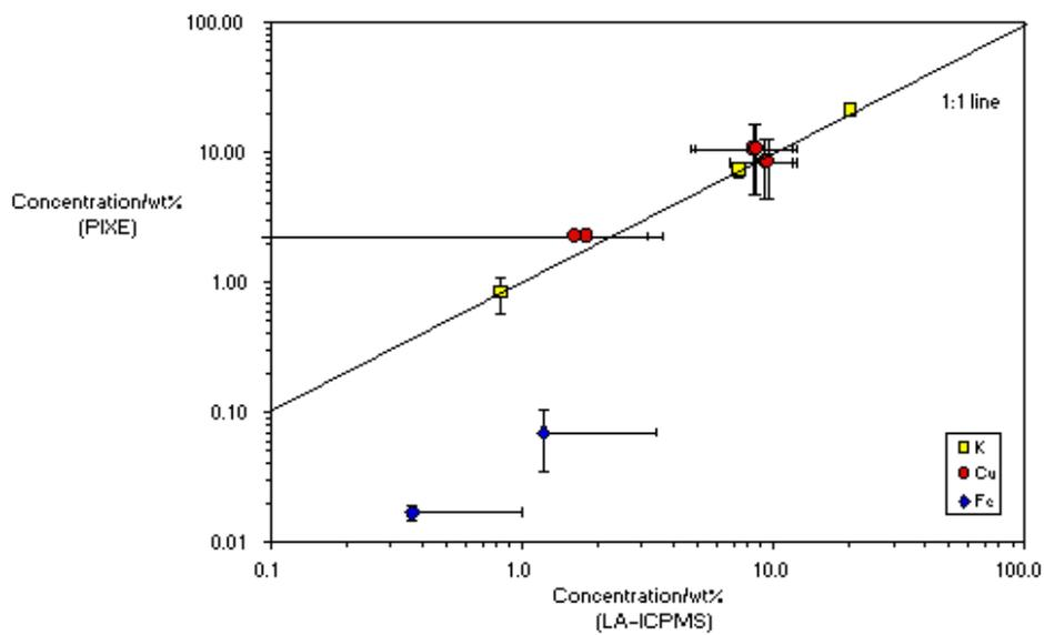
*Figure 1:* Comparison of LA—ICPMS and PIXE synthetic fluid inclusion data from three experiments at different run conditions for Cu, K, and Fe. LA—ICPMS data were quantified by using the K concentration determined by PIXE as an internal standard and NIST 612 silicate glass as the external analytical standard. Errors = 1s.
