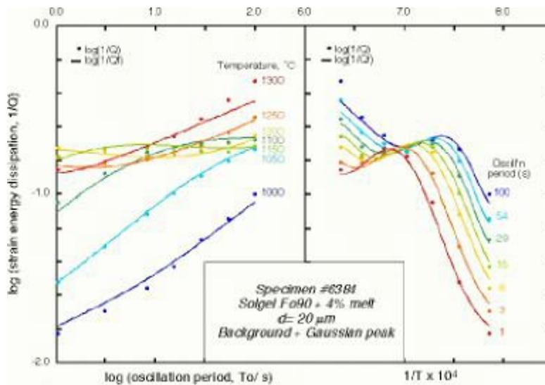
Figure 7 The variation of strain energy dissipation with oscillation period and temperature for specimen #6384 (sol-gel  $FO_{90}$  + 4% basaltic melt). Data are indicated by the plotting symbols, whereas the curves represent a fit to the data involving superposition of a Gaussian dissipation peak upon the monotonic background characteristic of melt-free materials.
