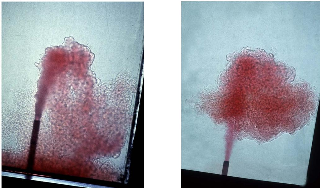
*Figure 2:* Photographs of turbulent axisymmetric fountains formed from a source inclined at 10 degrees to the vertical, in a homogeneous fluid (left), and in a stratified fluid, for the limiting case of zero buoyancy flux at the source (right).
