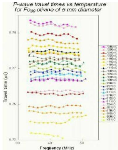
Representative data from ultrasonic interferometry illustrating the redundancy provided by traveltime determination from multiple interference minima.
