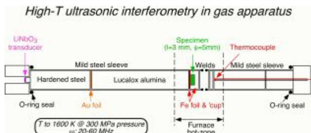
Experimental assembly for measurement of the temperature dependence of elastic wave speeds in an internally heated gas-charged pressure vessel by ultrasonic interferometry.
