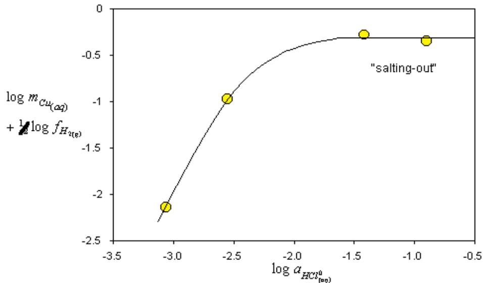
Figure 2: Thermodynamic representation of the copper solubility data with respect to reaction 1. Curve fit by eye.
