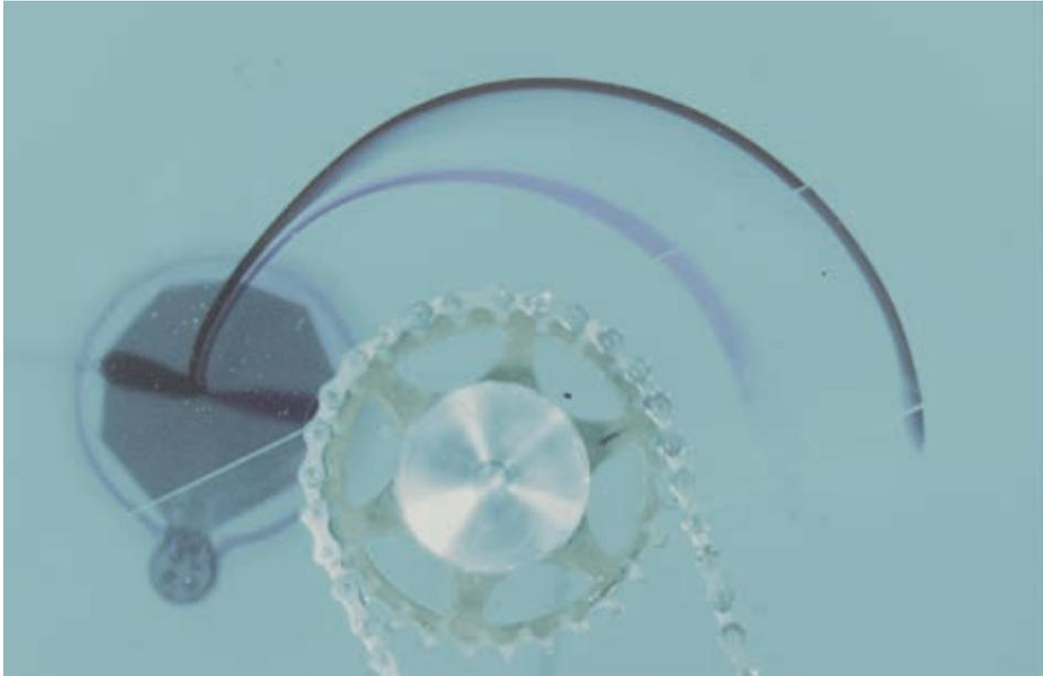
*Figure 7:* View from the top of a steady tilted plume conduit in a shear flow. Two streams of dyed glycerol are entrained into the plume within the heated bottom boundary layer (Rayleigh number  $1.4 \times 10^{10}$  and velocity ratio 0.4).
