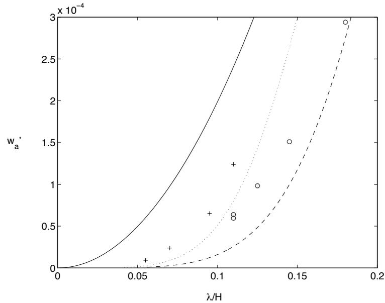
*Figure 6:* Comparison of theoretical predictions and experimental measurements for strongly damped internal gravity wave fields. The dimensionless vertical phase velocity  $w'_a$  of a wave mode is plotted as a function of dimensionless vertical wavelength  $\lambda/H$ : ——— inviscid theory; + and O, experimental measurements for two different levels of damping; ······ and - - - - , damped theory corresponding, respectively, to the two levels of damping.
