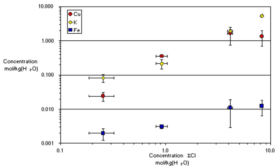
*Figure 1:* Solubility data for Cu, K, Fe in moles per kilogram H<sub>2</sub>O at 700°C and 300MPa as a function of total chlorine measured in individual quartz-hosted fluid inclusions by LA—ICPMS and PIXE. Fluid was buffered by the mineral assemblage quartz-sillimanite-K—feldspar-magnetite-hematite. Errors = 1s
