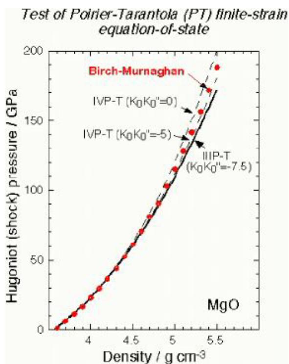
Figure 9 Comparison of calculated Hugoniots for MgO based on the alternative Eulerian and Poirier-Tarantola isentropes. The Hugoniot based on the 3rd-order Poirier-Tarantola isentrope is clearly too compressible at very high pressure.
