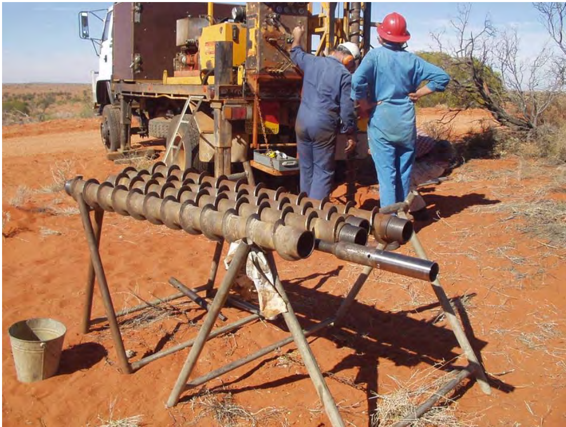
Figure 2. Drilling large longitudinal dunes in the Simpson Desert, for Optically Stimulated Luminescence and cosmogenic nuclide dating
