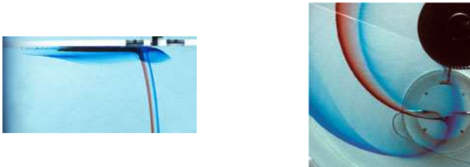
Figure 4: Front and overhead views of a weakly sheared thermal plume, with a high viscosity ratio (see also Figure 3).
