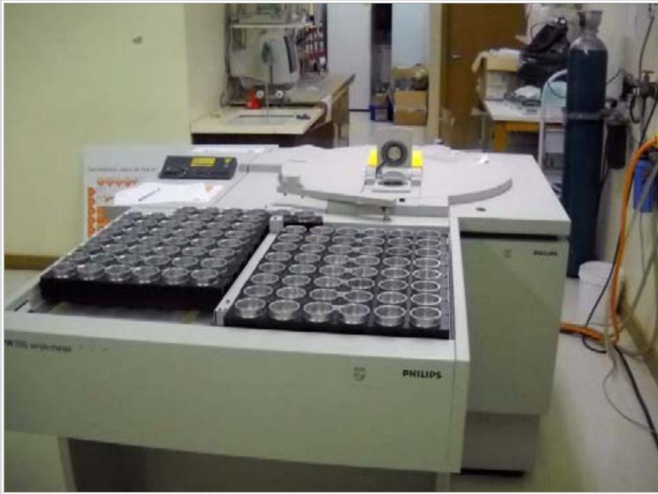
*Plate 5.5 XRF analyser with modern automatic sample changer*
