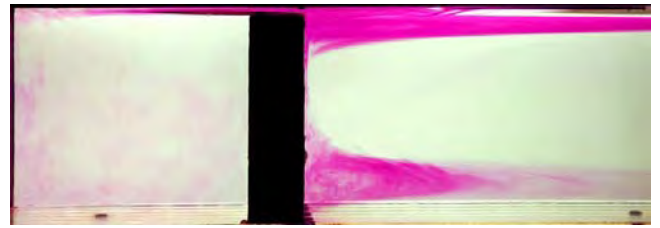
Figure 1. Dye visualization of a horizontal convection experiment with a large topographic sill (the field of view includes only the left-hand half of the box). The overturning circulation is forced by surface cooling at the left-hand end of the box ("polar latitudes") and surface heating over the right-hand end ("equatorial latitudes"; not visible). The circulation is in thermal equilibrium. The dye originates at the surface at top right of the tank and marks relatively warm surface water flowing from right to left towards the sill, where some of it mixes with dense water overflowing the sill (from the smaller basin on the left) and sinks to the bottom in the overflow plume. This "short-circuiting" within the main basin warms the deep water in that basin.
