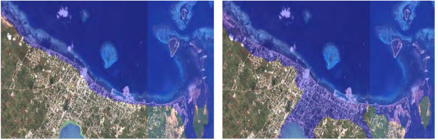
Figure 2. Tsunami inundation modelling results for a magnitude 8.25 scenario earthquake on the Tonga Trench, compared using two different bathymetry models: (left) a previous model obtained using an empirical method with 30 m Landsat data, and; (right) a new model obtained using a physics-based approach (SAMBUCA) with 2.4 m QuickBird data.
