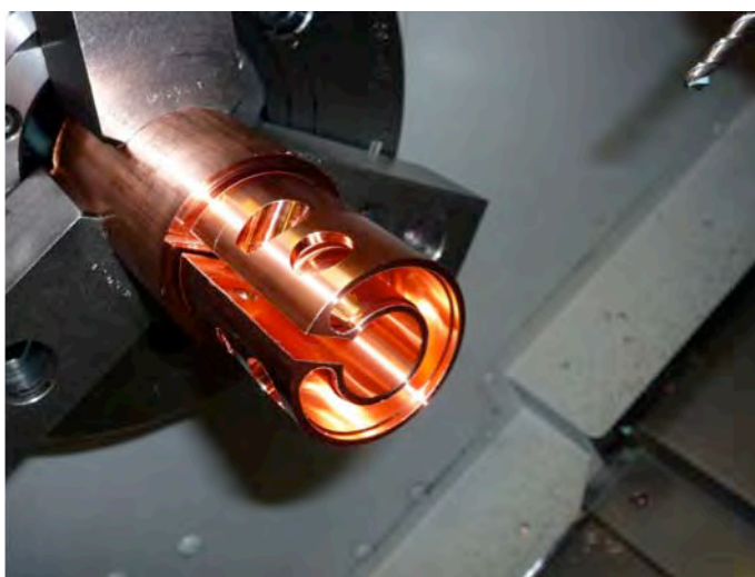
Water cooled electrical coupling used on Noble gas high temperature furnace
