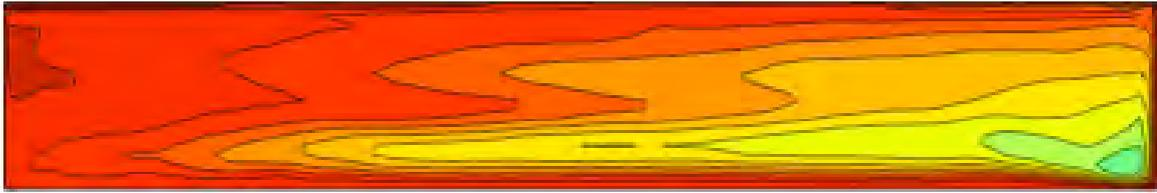
Figure 2. The stream function from a numerical simulation of the experiment in figure 1. The black contour lines represent streamlines of the flow; close contour lines mean faster flow velocities.
