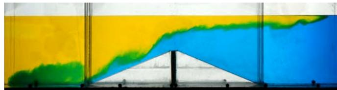
Exchange flow over a sill in the laboratory, showing shear instability and mixing.
