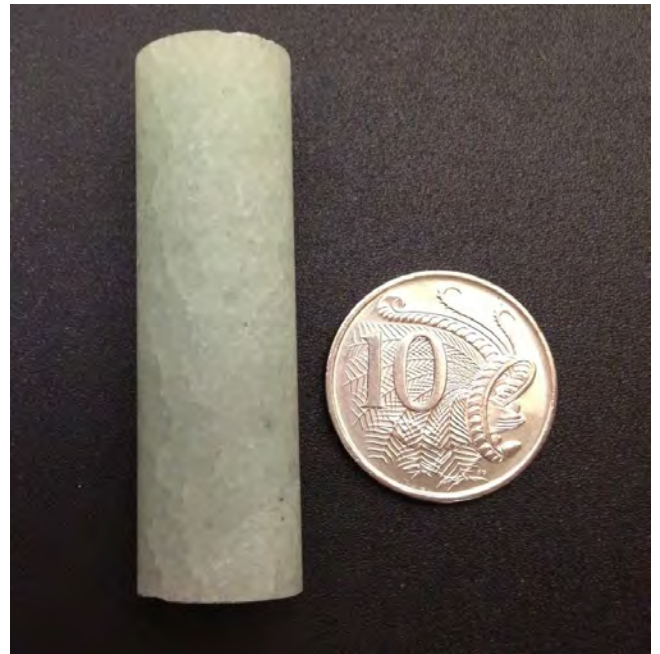
Figure 1. The glassbead specimen after thermal cracking with 15 mm diameter and 50 mm length.
