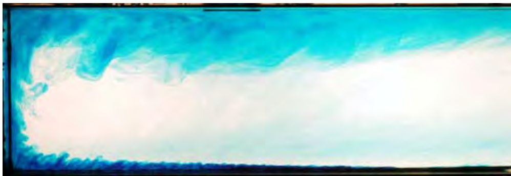
Figure 1: A photograph of dye tracer in the convective circulation in a long box of water which is cooled through the right hand half of the base and heated through the left hand half of the base. The box interior is 1.25 m long and 0.2 m high, but only the left 1/2 of the length is shown. Features include small-scale convection above the heated base of the tank, with a narrow plume ascending on the left hand wall.
