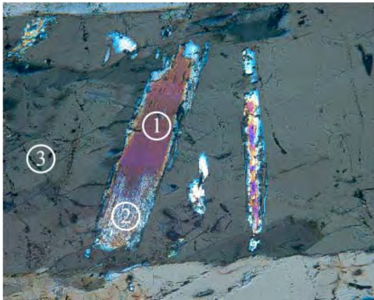
Figure 3. Photograph of a retrogressed eclogite under crossed polarizers. The oldest amphibole (1) breaks down in an albite+actinolite simplectite (2). Both (1) and (2) are then included in a large younger amphibole (3)
