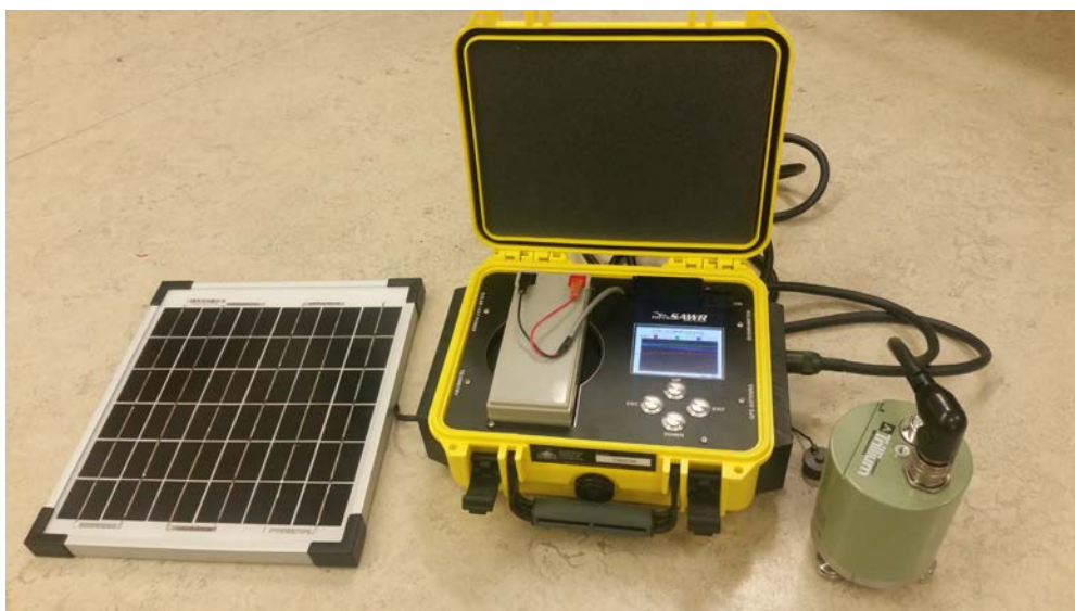
Fig 3. TerraSAWR seismic recording system with solar array and seismograph sensor
