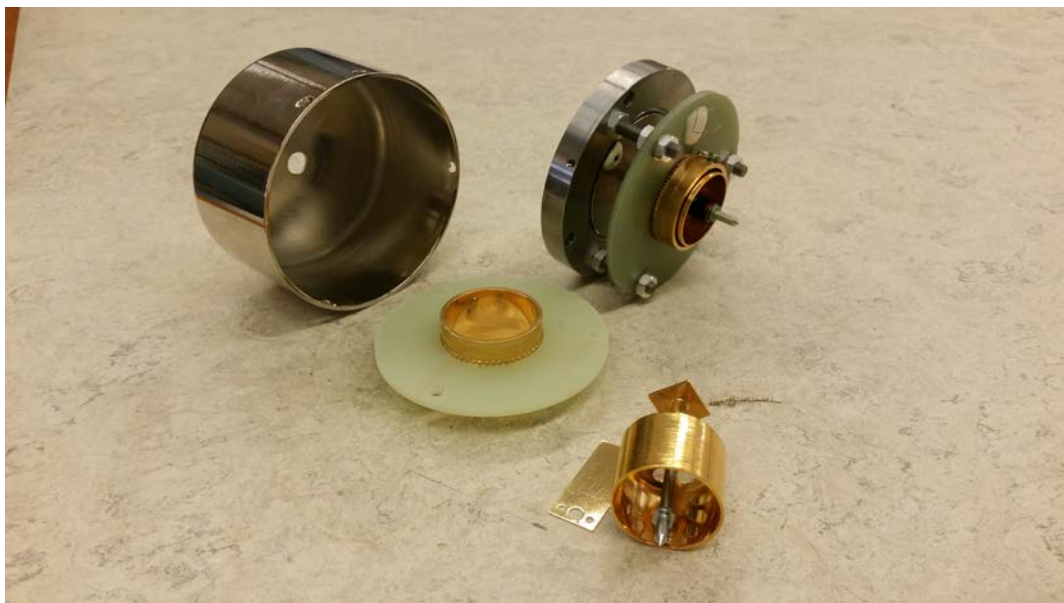
Fig 2. RSES-built vibrating reed, vacuum gap, variable capacitor
