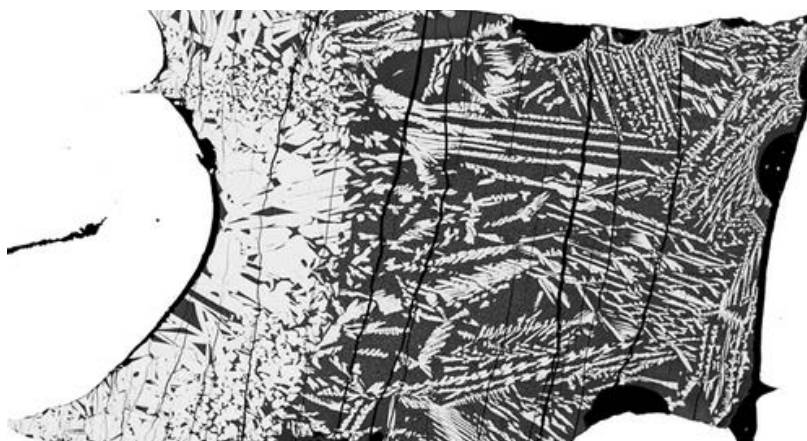
A back-scattered electron image of a high pressure experimental run showing primary and quench monazite crystals in a quenched carbonate-phosphate melt. Courtesy Srijita Ray, PhD student in Experimental Petrology.
