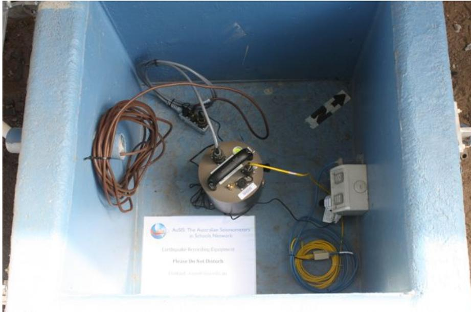
Figure 2. Installation at Ayr State High School. The Seismic Vault was built by students in the construction class.
