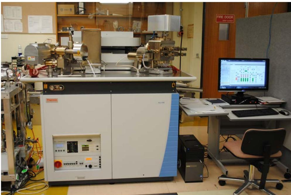
Figure 1. Helix-MC multi-collector noble gas mass spectrometer installed at RSES.
