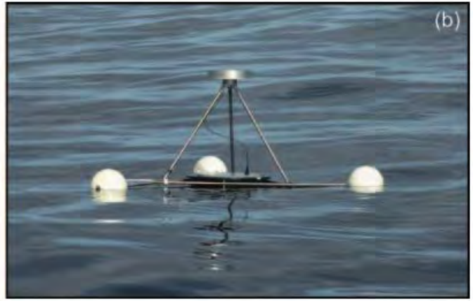
Figure 3. Floating GPS buoys used to measure directly the height of the sea surface in Bass Strait (Watson et al., 2011)
