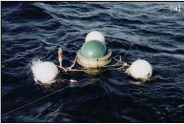
Figure 3. Floating GPS buoys used to measure directly the height of the sea surface in Bass Strait (Watson et al., 2011)
