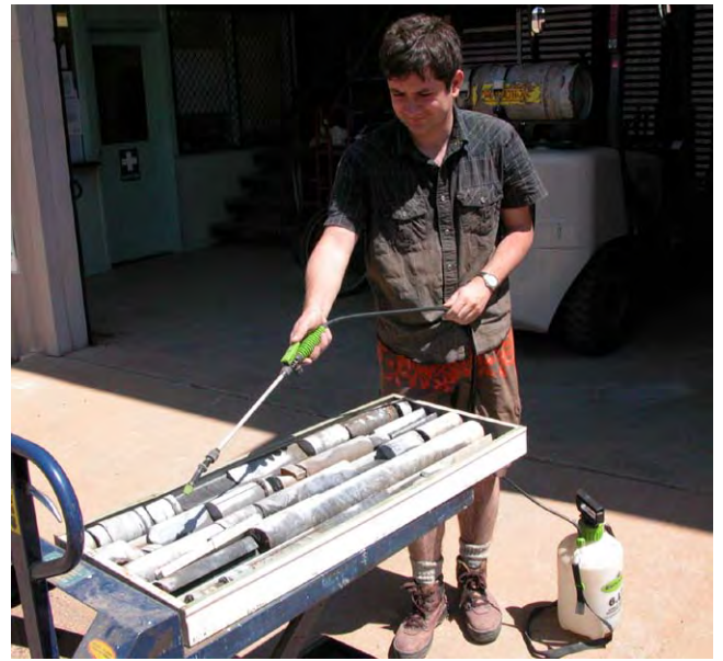
Figure 1. PhD Student Richard Schinteie sprays 800 million year old, carbon-rich carbonates with diesel oil: "This is the only way to find steranes in these ancient rocks", he justifies his action
