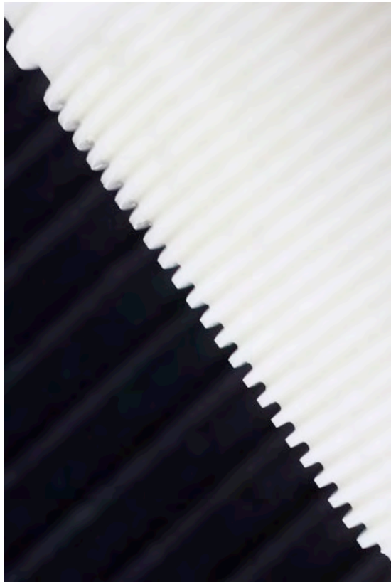
Rock Mechanics Furnace Core- Showing fine helical grooving in Aluminum Oxide for heater windings
