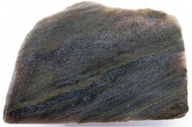
Figure 1. Example of an evaporitic sample from which lipid biomarkers were extracted. The sample is composed of grey-brown dolomitic laminae and gray-white crystalline anhydrite. Sample is 7 cm wide.
