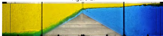
Figure 3. Dye visualizations of exchange flow experiments. Fresh water (yellow) flows from left to right and salt water solution (blue) from right to left. Exchange takes place through a pure lateral constriction (situated between the two bands of vertical lines) in the first case, and across a bottom sill located in the constriction in the second case. The third case shown has a higher topographic sill and a larger Reynolds number. Strong interfacial disturbances lead to turbulence and mixing.
