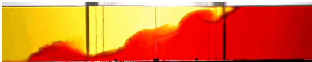
Figure 1. Shear instability and mixing in an hydraulically-controlled exchange flow through a short constriction.
