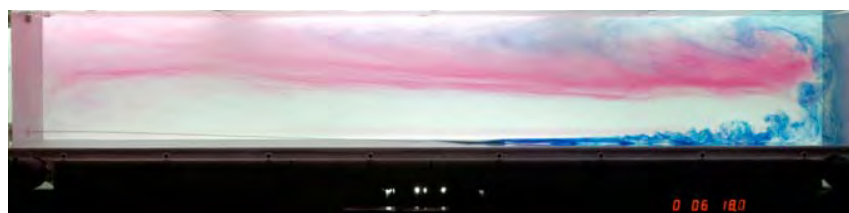
Figure 1. A photograph of dye in the convective overturning when a larger heat flux is applied to the left hand side of the base of a box, a weaker heat flux is applied to the right hand side of the base, and the central section of the base is cooled such that there is no net heat input. In this example the right hand plume drives a shallow cell, and its water (blue) is eventually entrained into the stronger plume at left and cycled throughout the box.
